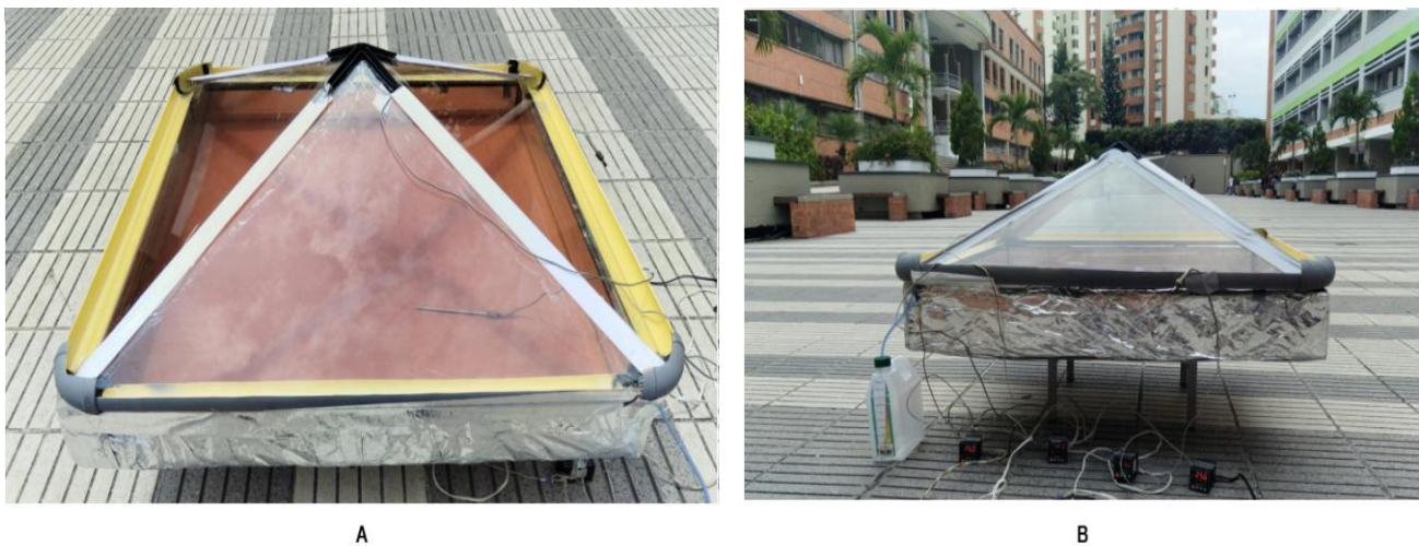
Figure 3. Side view (A) and low-angle view (B) of the pyramidal solar distiller built according to the concept of appropriate technology
