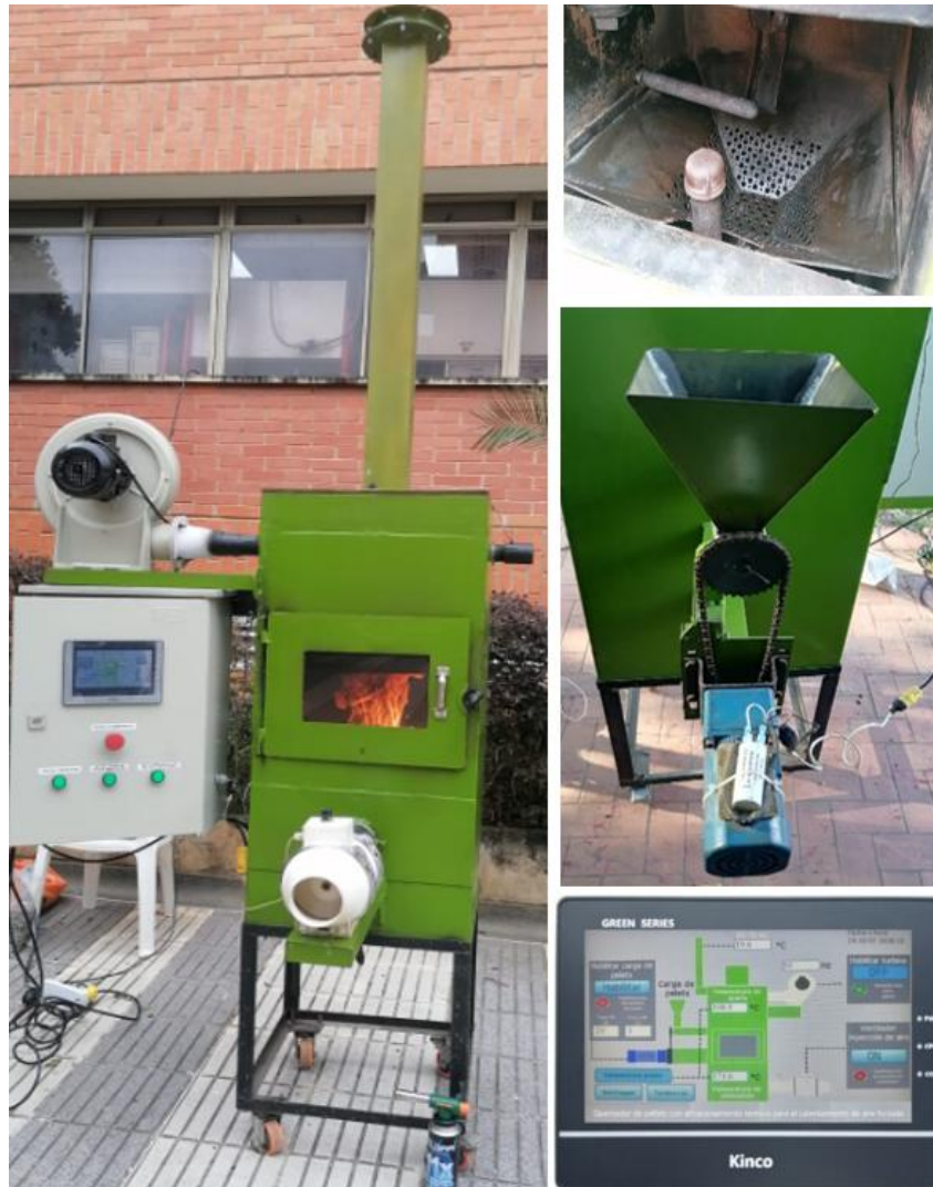
Figure 5. Burner equipment, perforated basket, pellet hopper, and HMI screen
